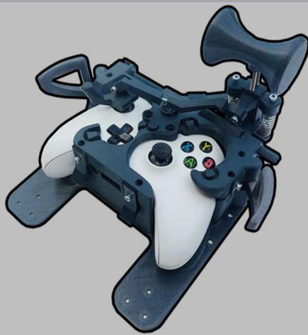
Figure 1: The third version of the adaptive gaming controller add-on
