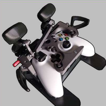
Figure 2: The second version of the adaptive gaming controller add-on and a video of Levente using it for the first time
